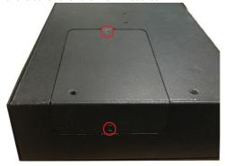
2. Remove the cover to access the SD-card slot and the mSATA  $\,$  mSATA
