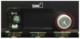
Insert the SIM card into the slot. Make sure you insert the card in the direction indicated above the card slot.
