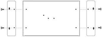
These four screws are included in the wall-mounting kit. Refer to the right figure for the detailed specifications.
