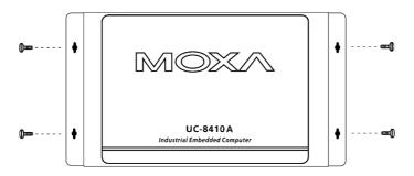
These four screws are not included in the wall-mounting kit and must be purchased separately. Refer to the detailed specifications on the right. **Head Type:** round or pan **Head Diameter:** > 4.5 mm
