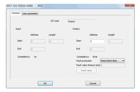
For some applications, you may want to define how to deal with the PROFIBUS output when the Modbus TCP side is not working properly. This is defined as the "Fault value". The MGate provides a setting for each PROFIBUS I/O module to handle this kind of situation.
