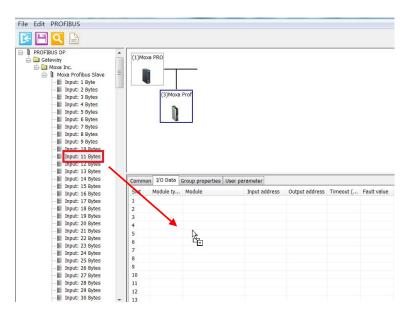
The added I/O device will appear in the lower portion of the right panel.
