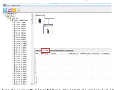
Drag the proper I/O module from the left panel to the right panel to complete the configuration.
