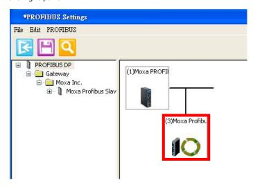
To remove the device from the PROFIBUS network (depicted at the top of the right panel in the figure above), right-click on the device and select **Delete device** or directly press the DELETE button on your keyboard.
