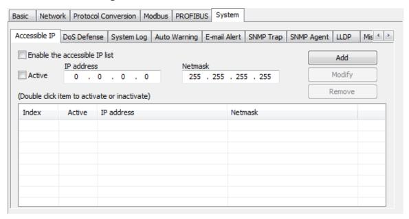
These settings are used to restrict access to the module by IP address. Only IP addresses on the list will be allowed access to the module. You may add a specific address or range of addresses by using a combination of IP address and netmask, as follows:
