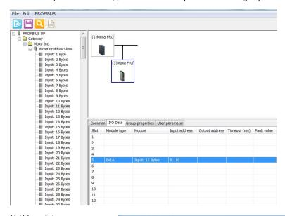
At this point, you can configure device parameters, including the slave address and I/O modules. To configure each I/O module in detail, double click the I/O module to display the configuration dialog. In the dialog box, configure the internal memory address Offset and Fault values. To configure these parameters, refer to the Data Exchange Between PROFINET and PROFIBUS and Fault Value Configuration in the PROFIBUS Output Module sections.
