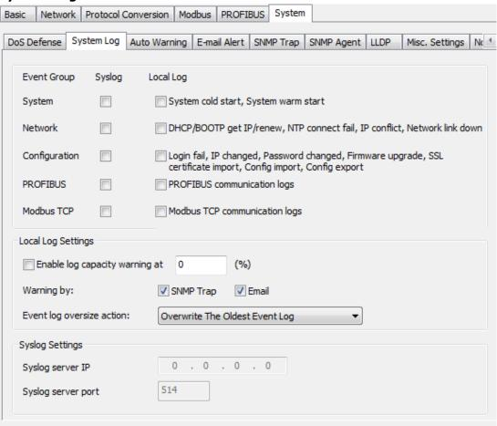
This setting will enable the MGate firmware to record important events for future verification. The recorded information can only be displayed in the web console. See Chapter 5 for details.
