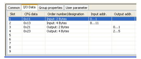
With the following example, if user wants to access bit 1 of the input address 1. The users have to use the [01-read coil] command to read the address = 1\*8+1+1=9. If users want to access the 4 bytes input data with Modbus register access command, the users have to use the [03-read holding register] command to read the address = 8/2+1=5 with length 2.
