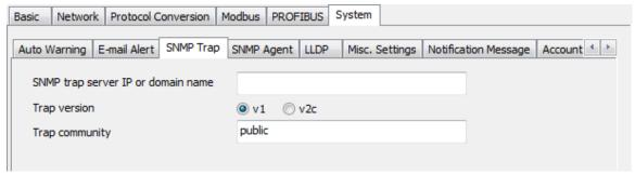
The MGate gateway supports Simple Network Management Protocol (SNMP).
