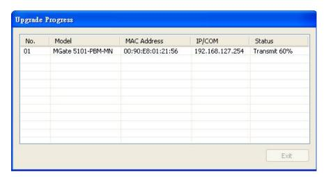
Once the firmware has been successfully written to the unit, click **Exit** to close the Upgrade Firmware window. MGate Manager will automatically execute a Broadcast Search to all MGate units on the LAN. Your MGate should reappear in the list of units.
