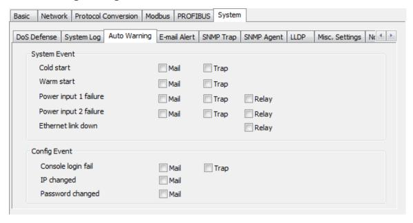
Auto Warning will be triggered in the event of a power failure or when Ethernet links are disconnected. When a checked trigger condition occurs, the MGate will open the circuit of the relay output. To enable an email alert, configure the e-mail address on the E-mail Alert page. Likewise, to enable SNMP Trap alerts, configure SNMP trap server on the SNMP Trap page.
