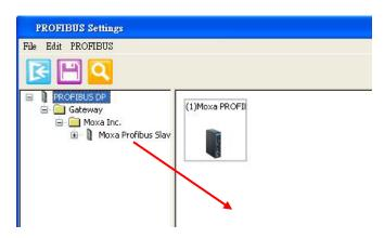
To add the device to the PROFIBUS network shown in the right panel above, drag the device from the left panel and drop it into the right panel. The device will then be shown beneath the network icon depicted in the right panel.
