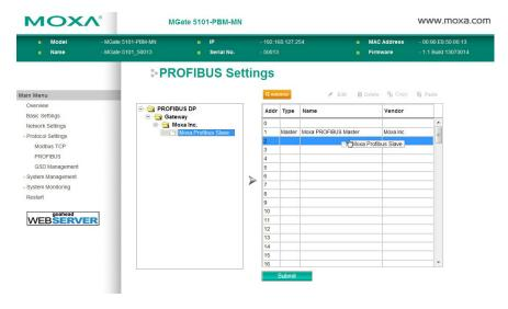
After you add the device to the MGate gateway, click the **Edit** button to edit related settings. See **PROFIBUS Settings** in Chapter 4 for a description of each function.
