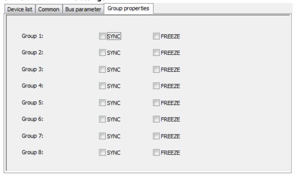
SYNC: In data\_exchange the previous output value will be transferred. The following output data will be stored and not be transferred until next SYNC command or UNSYNC command.
