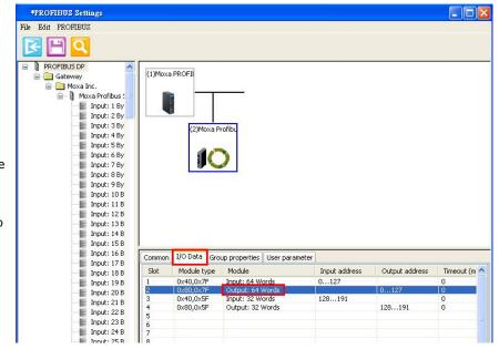
To remove the I/O modules, select the I/O module and right-click  $\bf I/O$  module and select  $\bf Delete\ I/O$  or directly press the DELETE button on your keyboard.
