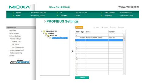
To add a device to the MGate gateway, drag the slave device to the list on the right side.
