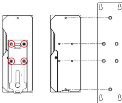
**STEP 2**—Mounting the EDS device on a wall requires four screws. Use the EDS device, with wall mount plates attached. The heads of the screws should be less than 6.0 mm in diameter, and the shafts should be less than 3.5 mm in diameter, as shown in the figure on the right.
