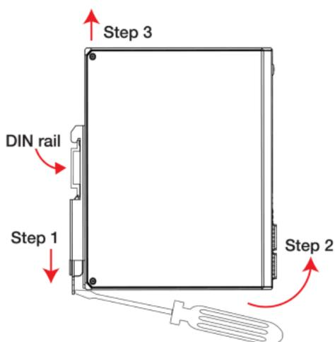
**NOTE** Our DIN rail kit now utilizes a quick release mechanism to make it easier for users to remove the DIN rail from the EDS device.
