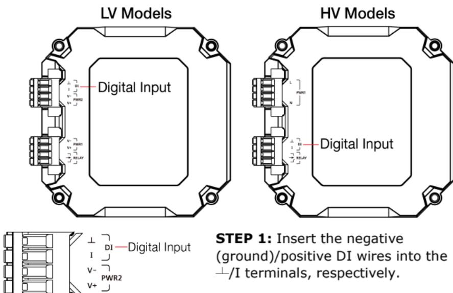
**STEP 1:** Insert the negative (ground)/positive DI wires into the  $\perp$ /I terminals, respectively.
