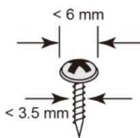
**NOTE** Before tightening the screws into the wall, make sure the screw head and shank size are suitable by inserting the screw through one of the keyhole-shaped apertures of the Wall Mounting Plates.
