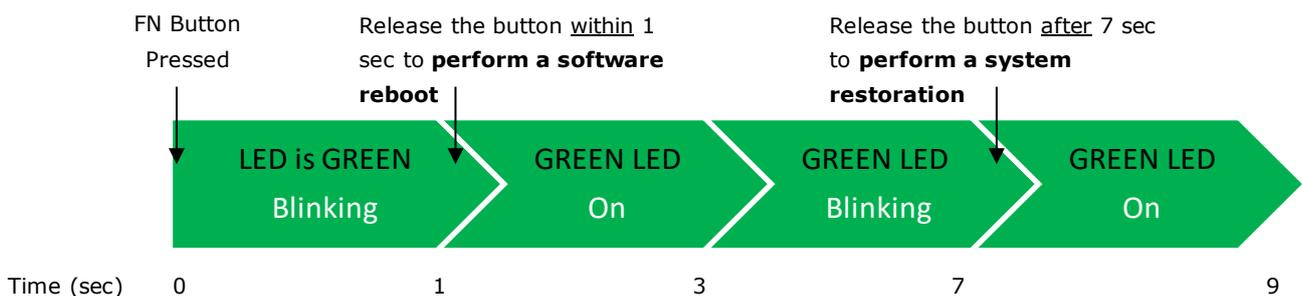
The mapping of the action on the FN button with the behavior of the SYS LED and the resulting system status is given below:
