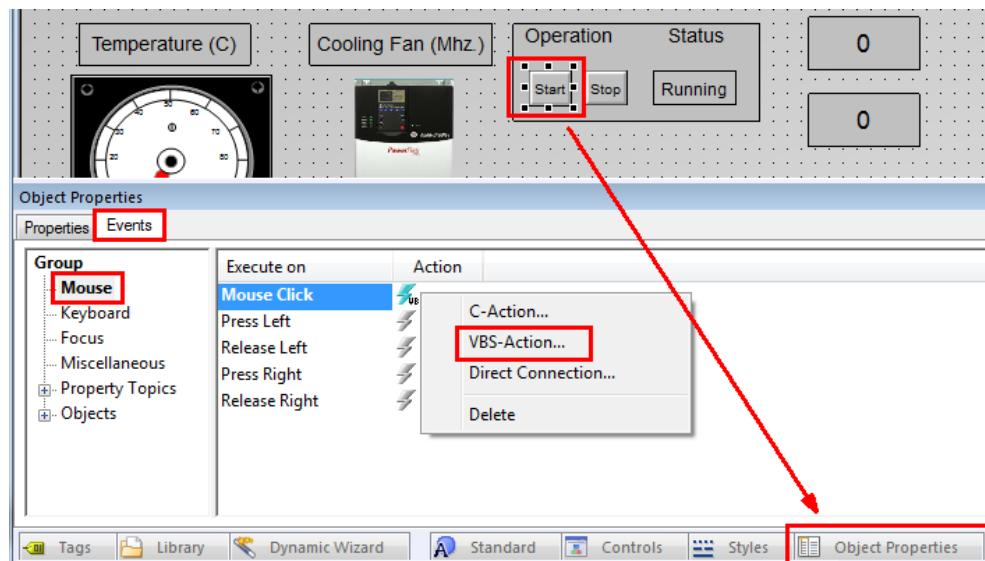
The script program appears as shown in the following figure. The script sets the value of the **byModbus** tag to "1" when the **Start** button is clicked.
