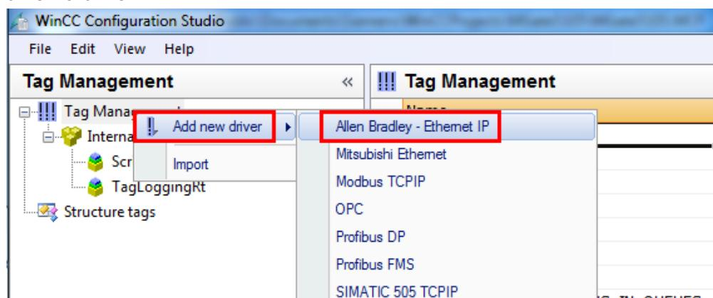
The WinCC Configuration Studio screen displays the **Allen Bradley – Ethernet IP** channel that you have added. The Allen Bradley – E/IP ControlLogix channel provides several channel units for different communication networks.
