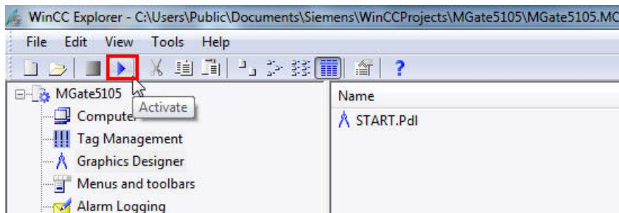
The system starts Graphics Runtime and the **START.pdl** process picture is displayed as the startup screen.
