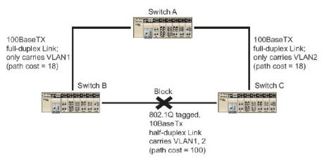
To avoid subdividing VLANs, all inter-switch connections should be made members of all available 802.1Q VLANs. This will ensure connectivity at all times. For example, the connections between Switches A and B, and between Switches A and C should be 802.1Q tagged and carrying VLANs 1 and 2 to ensure connectivity.
