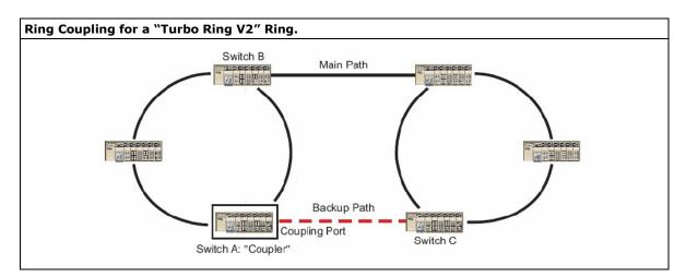
Note that the ring coupling settings for a "Turbo Ring V2" ring are different from a "Turbo Ring" ring. For Turbo Ring V2, Ring Coupling is enabled by configuring the "Coupling Port (Primary)" on Switch B, and the "Coupling Port (Backup)" on Switch A only. You do not need to set up a coupling control port, so that a "Turbo Ring V2" ring does not use a coupling control line.
