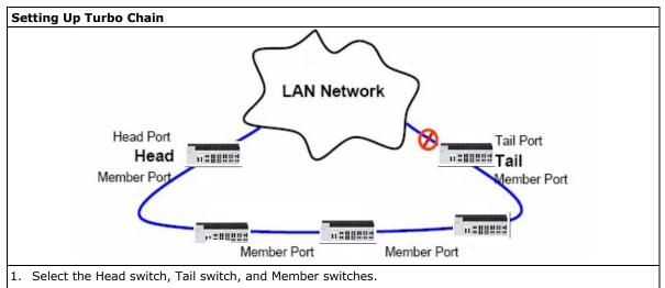
2. Configure one port as the Head port and one port as the Member port in the Head switch, configure one port as the Tail port and one port as the Member port in the Tail switch, and configure two ports as Member ports in each of the Member switches.
