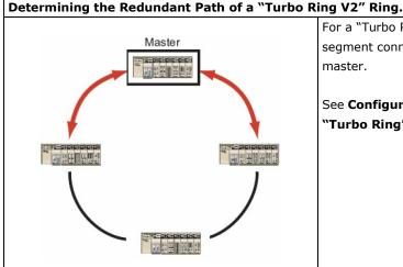
For a "Turbo Ring V2" ring, the backup segment is the segment connected to the 2nd redundant port on the master.
