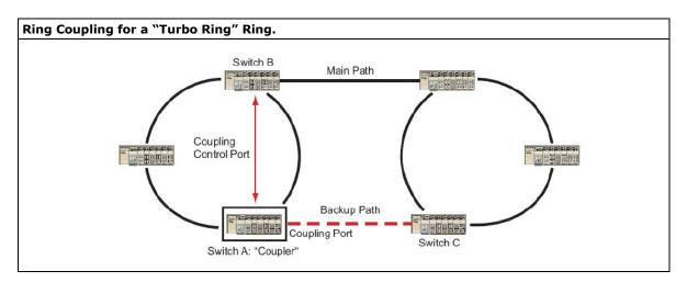
To configure the Ring Coupling function for a "Turbo Ring" ring, select two EDS-728 units (e.g., Switch A and B in the above figure) in the ring, and another two EDS-728 units in the adjacent ring (e.g., Switch C and D).
