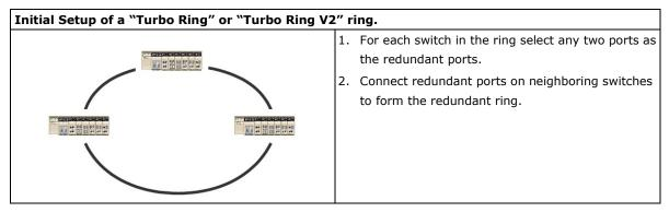
The user does not need to configure any of the switches as the master to use Turbo Ring or Turbo Ring V2. If none of the switches in the ring is configured as the master, then the protocol will automatically assign master status to one of the switches. In fact, the master is only used to identify which segment in the redundant ring acts as the backup path. In the following subsections, we explain how the redundant path is selected for rings configured for Turbo Ring, and Turbo Ring V2.
