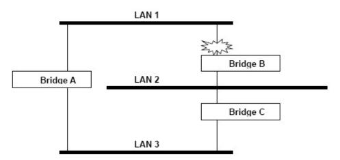
What happens if a link failure is detected? As shown in next figure, the STP process reconfigures the network so that traffic from LAN segment 2 flows through Bridge B.
