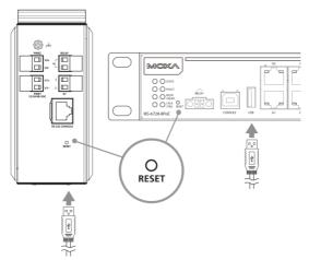
The "RESET" button is located on the front panel of rackmount type switches and on the top panel of DIN-rail type switches.
