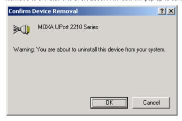
3. Click **OK** to continue uninstalling the UPort device. The UPort device will be removed from the list of **Multi-port serial adapters**.
