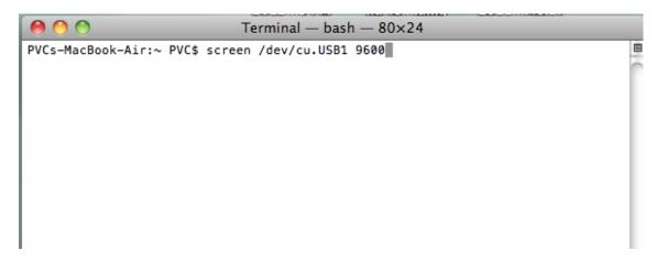
Data entered in the terminal emulator for serial port 1 will be displayed on the terminal emulator for serial port 2, and vice versa. The LEDs will blink as you type, showing that data is being transmitted and received between the two serial ports.
