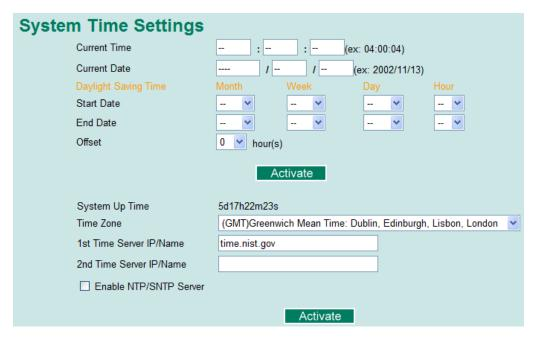
The Moxa switch has a time calibration function based on information from an NTP server or user specified time and date. Functions such as automatic warning emails can therefore include time and date stamp.
