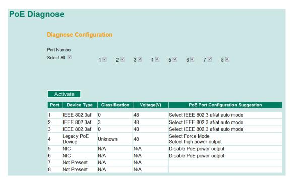
**PoE Diagnose** helps users to figure out the PD conditions, and the system provides users configuration suggestions to select the best setting for the PDs.
