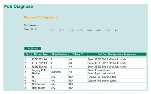
**PoE Diagnose** helps users to figure out the PD conditions, and the system provides users configuration suggestions to select the best setting for the PDs.
