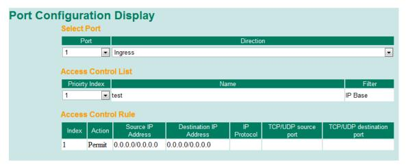
**NOTE** For TN-5800A series, there are two limitations on ACL settings. Based on the ingress port type of ACL rules, there are two types for the limitation of numbers.
