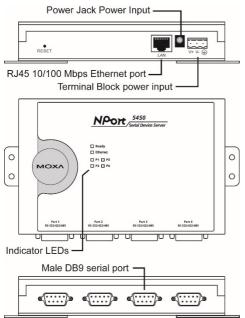
**Reset Button**—<u>Press the Reset button continuously for 5 sec to load</u> <u>factory defaults:</u> Use a pointed object, such as a straightened paper clip or toothpick, to press the reset button. This will cause the Ready LED to blink on and off. The factory defaults will be loaded once the Ready LED stops blinking (after about 5 seconds). At this point, you should release the reset button.
