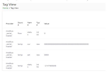
You can write a value to the Modbus via Direct Write Value to test the communication with Modbus device.
