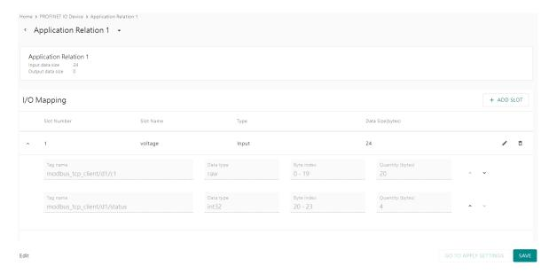
Click **ADD SLOT** in the I/O Mapping to add tag data to PROFINET slots.
