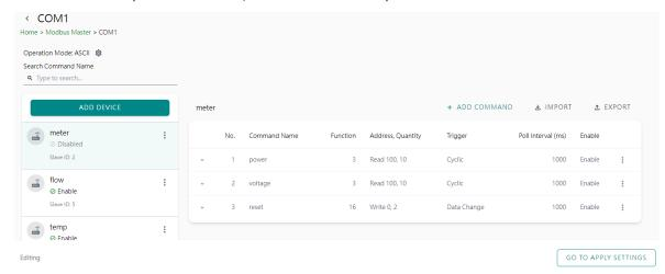
After configuring all Modbus TCP or Modbus RTU/ASCII settings, please remember to click **GO TO APPLY SETTING** and press the **APPLY** button at the bottom right-hand side corner.
