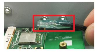
5. Connect the antenna cables to the antenna connectors. The Wi-Fi module supports two antenna connectors; connect the cables to the correct antenna connectors.
