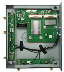
4. Install the cellular module onto the socket, and fasten the two screws on the module.
