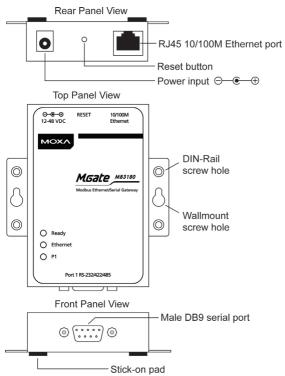
**Reset Button**—The reset button is used to load factory defaults. Using a pointed object such as a straightened paper clip to hold the reset button down for five seconds. Release the reset button when the Ready LED stops blinking in order to load the factory defaults.
