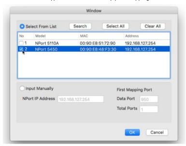
7. NPortConnect would auto assign the tty name and corresponding port number to the IP address of the selected NPort.
