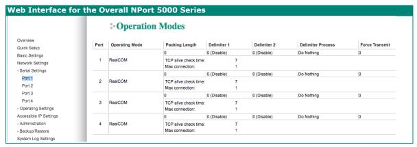
For each mode, the default settings should work for most applications. Modify these settings only if absolutely necessary for your application. The operation mode and related parameters can be configured through the web console. The same parameters can also be configured using NPort Administrator, the Telnet console, or serial console. Refer to **Chapters 4 and 5** for details.
