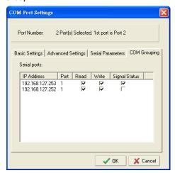
5. Click **OK**, and confirm that the serial ports that were assigned. The COM Port column confirms that your selected ports are labeled as part of a "Group." You will be able to view the serial ports that were assigned to and removed from the Group. Click **Apply** to apply the settings.
