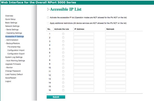
**Accessible IP Settings** allow you to add or block remote host IP addresses to prevent unauthorized access. Access to the NPort is controlled by an IP address. That is, if a host's IP address is in the accessible IP table, then the host will be allowed to access the NPort. Three setting types are described below:
