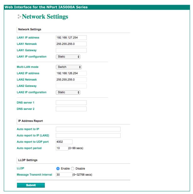
You must assign a valid IP address to the NPort before it will work in your network environment. Your network system administrator should provide you with an IP address and related settings for your network. The IP address must be unique within the network (otherwise, the NPort will not have a valid connection to the network). You can choose from four possible **IP configuration** modes—Static, DHCP, DHCP/BOOTP, and BOOTP—located under the web console screen's IP configuration dropdown box.
