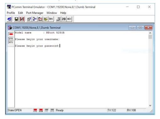
9. Start configuring the IP address under **Network Settings**. Refer to step 4 in the Telnet Console section for the rest of the IP settings.
