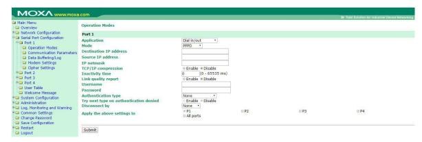
PPPD (PPP on demand) is used for dial-in services, since it provides PPP services only when receiving a request from a remote PC.
