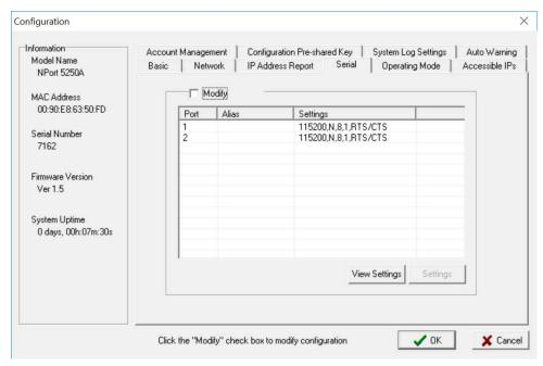
The serial communication parameters for each device port can be configured through NPort Administrator. Open your device server's configuration window, using the same method you used to configure network parameters. On the **Serial** screen, select the **Modify** check box and then select the device port you wish to configure. Click **Settings** to configure the selected device port.
