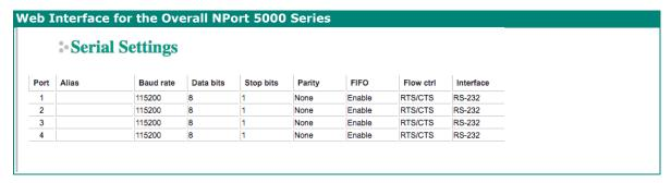
To modify serial settings for a particular port, click on the **Port Number** under **Serial Settings**, located under **Main Menu** on the left side of the browser window.
