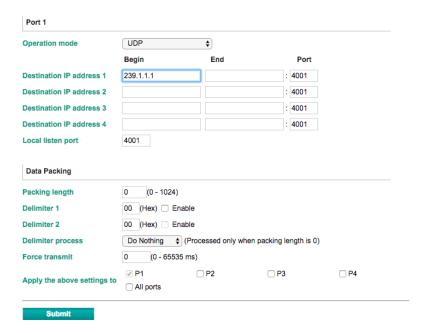
Type the IP address (e.g., 239.1.1.1) assigned to the multicast group in the **Begin** column. The NPort will automatically add the Group, and receive all packets from this group as required by the multicast function.
