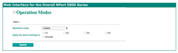
When Operation mode is set to Disabled, that particular port will be disabled. Select the **Apply the above settings to all serial ports** checkbox to apply this setting to the other ports.
