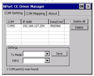
6. To configure the settings for a particular COM Port, select the row of the desired port, and then modify the setting in the "Settings" panel, as shown below.
