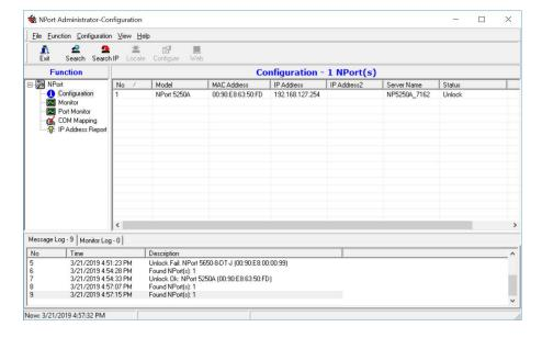
The **Configuration** screen will list the NPort device servers that were found on the LAN. If your unit cannot be found, you may have a network problem. Check all cables and verify that your PC and device server are on the same LAN. If you still have problems, try connecting the device server directly to your PC.
