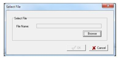
For the overall NPort 5000 Series with security enhanced firmware version, export configuration encryption will be based on the Pre-shared key defined in the NPort (default is empty password, and you may configure the password in **Configuration -> Configuration Pre-shared Key**. So when you are exporting the configuration file, you are only required to select the output file location. You may refer to page 2-21 for the security firmware version for your NPort.
