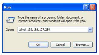
3. When the Telnet window opens, you will be prompted to input the Console password (the default username is **admin** and password is **moxa**; for the NPort 5100/5200/IA5000, it only requires the default password **moxa**); input the password and then press **Enter**.
