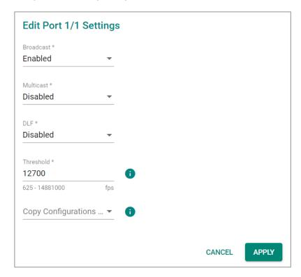
There are three methods that can be used for traffic storm control: Broadcast, Multicast, and Destination Lookup Failure (DLF).
