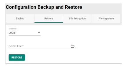
There are four ways to restore the configurations of your Moxa switch: from a local configuration file, by remote SFTP server, by remote TFTP server, or by a USB tool.
