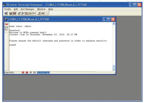
After successfully connecting to the switch by serial console, you can start configuring the switch's
