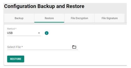
Insert Moxa's ABC-02 USB-based configuration tool into the USB port of the switch, click **RESTORE** to restore the system configuration file.
