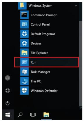
11. Next, use Telnet to connect the Moxa switch's IP address (192.168.127.253) from the Windows **Run** window. You can also issue the Telnet command from a DOS prompt.
