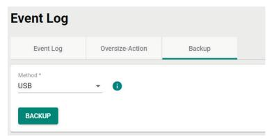
Insert a Moxa's ABC-02 USB-based configuration tool onto the USB port of the switch, click **BACKUP** to back up the event log files.
