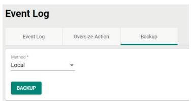
There are four ways to back up your event log files: from a local location of your computer, by remote SFTP server, by remote TFTP server, or by a USB tool.
