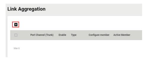
To create a link aggregation group, configure the following parameters.
