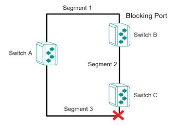
STP will determine which path between each segment is most efficient, and then assign a specific reference point on the network. When the most efficient path has been identified, the other paths are blocked. In the previous three figures, STP first determined that the path through switch C was the most efficient, and as a result, blocked the path through switch B. After the failure of switch C, STP re-evaluated the situation and opened the path through switch B.
