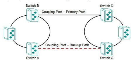
For Turbo Ring V2, Ring Coupling is enabled by configuring the **Coupling Port (Primary)** on Switch B, and the **Coupling Port (Backup)** on Switch A only.
