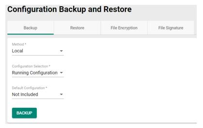
There are four ways to back up the configurations of your Moxa switch: from a local configuration file, by remote SFTP server, by remote TFTP server, or by a USB tool.
