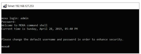
13. After successfully connecting to the switch by Telnet, users can start configuring the switch parameters by using command line instructions. Refer to the **Moxa Command Line Interface Manual**.
