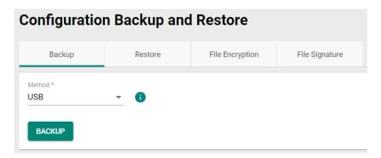
Insert Moxa's ABC-02 USB-based configuration tool into the USB port of the switch, click **BACKUP** to back up the system configuration file.
