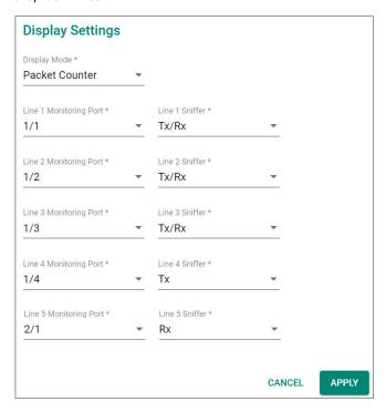
The Monitoring Port is the port you want to view or monitor. The sniffer port is the port that you can choose to view its receiving or transmission status or both.
