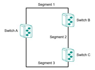
If STP is enabled, it will detect duplicate paths or block one of the paths from forwarding traffic. In the following example, STP determined that traffic from segment 2 to segment 1 flows through switches C and A since this path is in a forwarding state and is processing BPDUs. However, switch B on segment 1 is in a blocking state.
