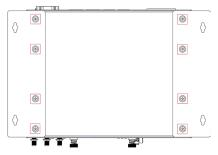
The screws are included in the wall-mounting kit. If you want to buy the screws separately, use the following specifications: Screw-M/FMS M4 x 6mm Ni/90D Nylok
