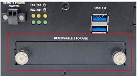
**Step 2:** Slide the latch on the disk tray to the left and pull out the tray from the slot.
