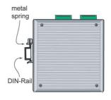
To remove EDS-505A/508A from the DIN-Rail, simply reverse Steps 1 and 2.
