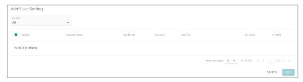
Or click the SCAN button to scan the device on the CAN bus. Only the slave device that matches the EDS file in the EDS Repository will be added to the table.
