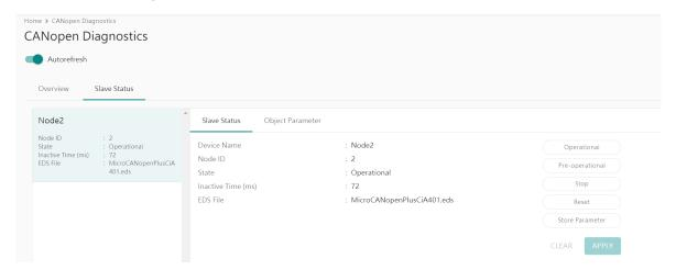
Furthermore, you can open the Object Parameter tab to check and change the slave device's CANopen object value.
