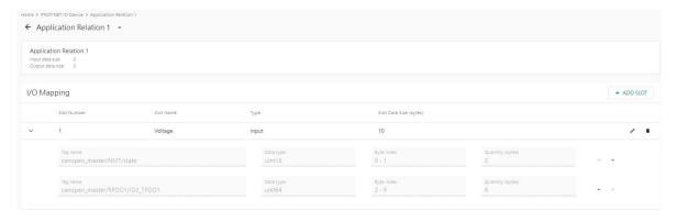
Click **ADD SLOT** in the I/O Mapping to add tag data to PROFINET slots.
