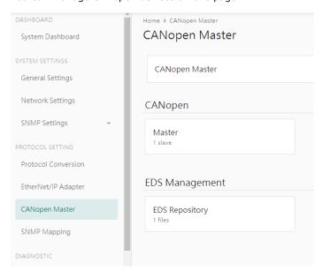
You can manage CANopen slave device EDS files in "EDS Management-EDS Repository". The MGate can store up to 64 different EDS files. Click Import to add the EDS file. Tick the item, then you can delete it.
