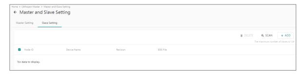
You can ADD slave device manually or SCAN the devices on the CANbus. Please import slave EDS files before adding or scanning the slave devices.
