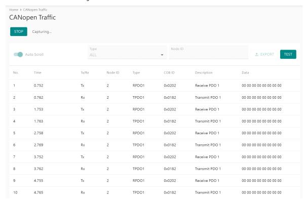
You can also read/write CAN data manually by clicking the TEST button and type in the CAN data frame.
